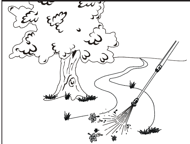
Figure 11 — Testing the Spray Pattern
